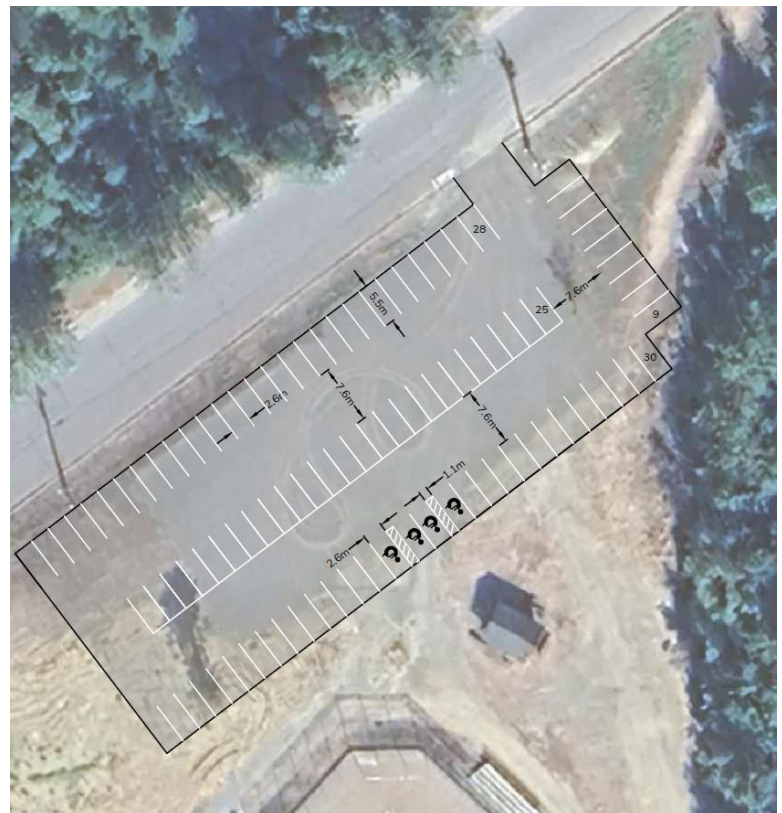
Figure 20: Potential Concept Design of Formalized Parking Lot at Point Ideal Sports Field
