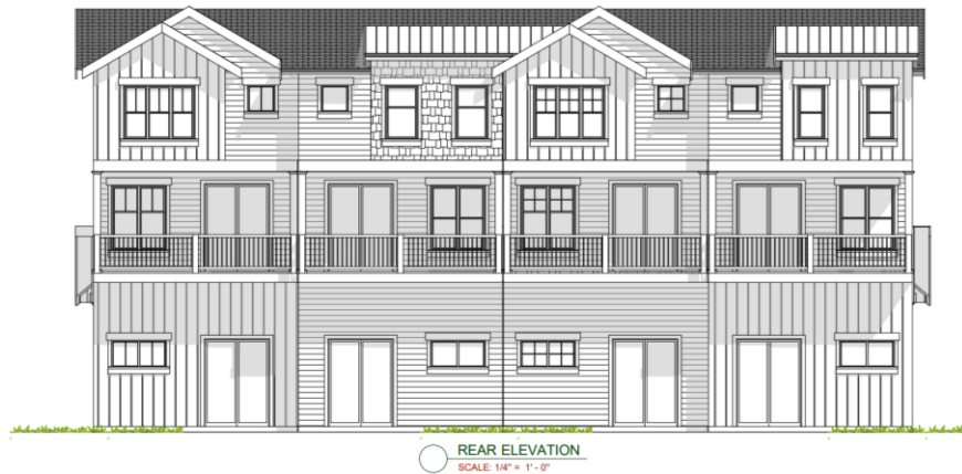
Figure 6 Rear elevation illustrating varied rooflines and materials
