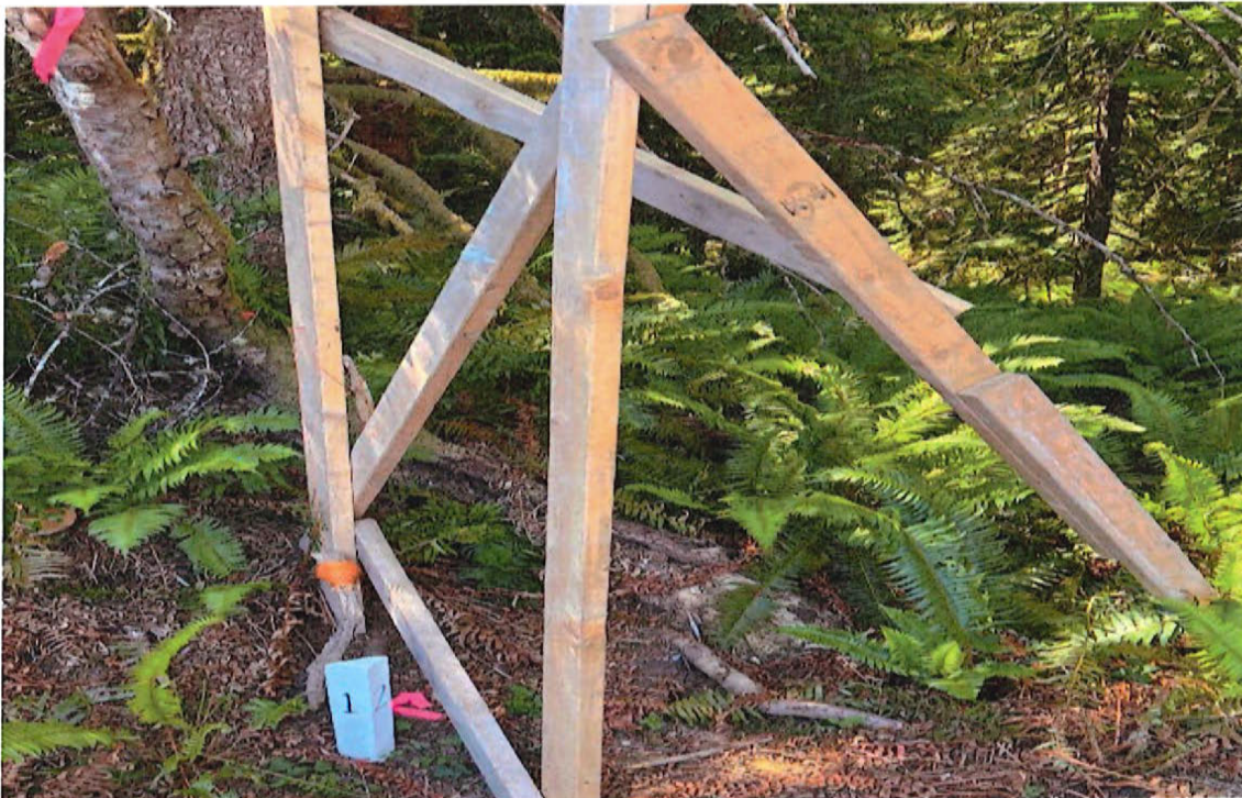
BCLS lot corner pin and guard/witness post for corner of Lot1 and Lot 2 (subject property).
